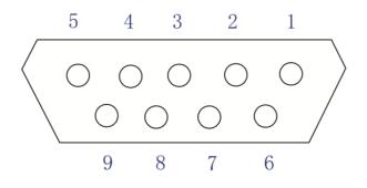
\*\*DB9 control pin description The port on the power supply board is the female connector. It needs to be equipped with a male connector to complete the corresponding control function.\*\*
